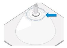
5. Apply the silicone slightly in from the outer edge on the underside of the basin.
